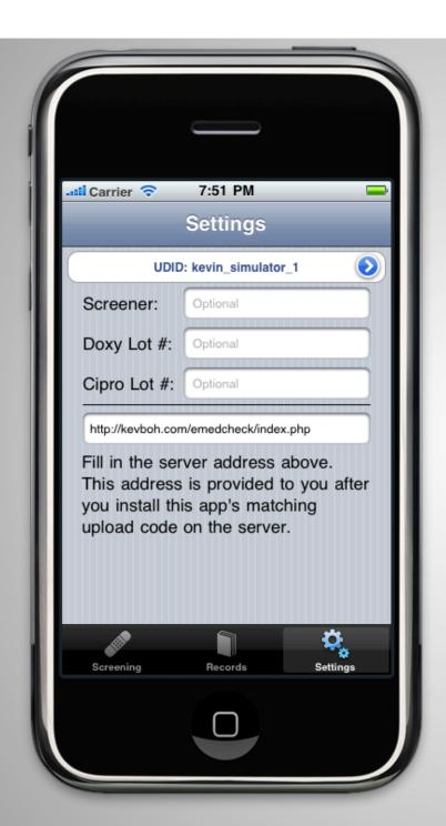
Settings provides a place to set the screener's name, lot numbers, our device's unique id (UDID), and our server's web address. You can see a test address in the bottommost text box- the .php tells us that we're sending our data to a php script, which will save it to our database. This address will always end in emedcheck/index.php
