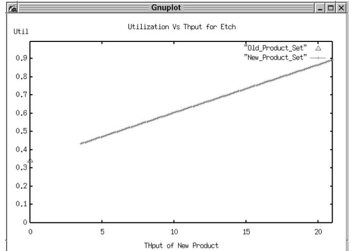
Figure 3: Machine Utilization as a function of New Product Throughput
