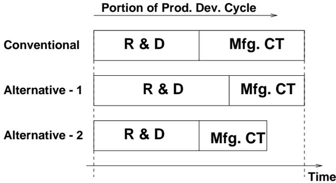
Figure 8: Lower manufacturing cycle time allows more time for research and development
