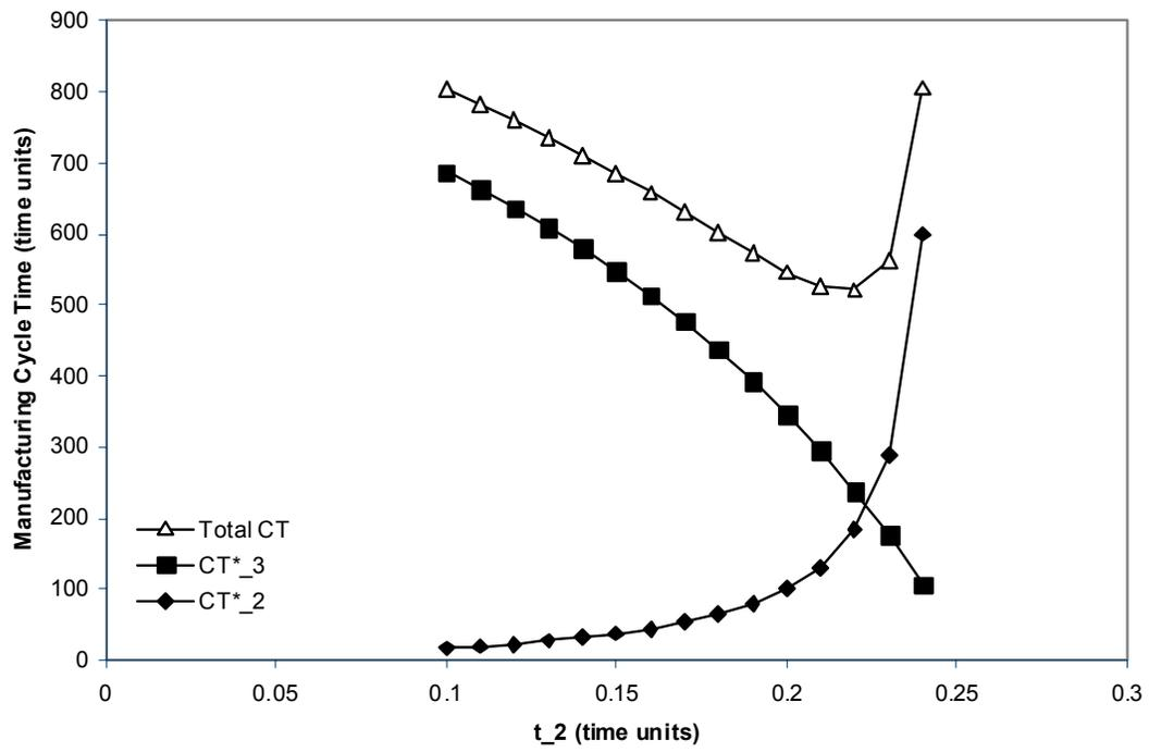
Figure 2. Manufacturing Cycle Time versus Part Processing Time.
