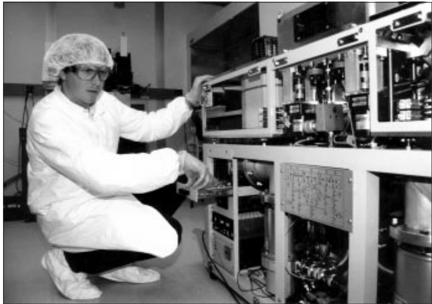
LAMP manager John Kidder operates the ERA-1000, housed inside a Class 1,000 Clean Room. Inside the two chambers of the ULVAC tool, a chemical vapor deposition process deposits tungsten metal film layers onto wafers by flowing gases at high temperatures (400 degrees Centigrade). A single wafer, holding 50–250 chips, can be processed in each chamber.
