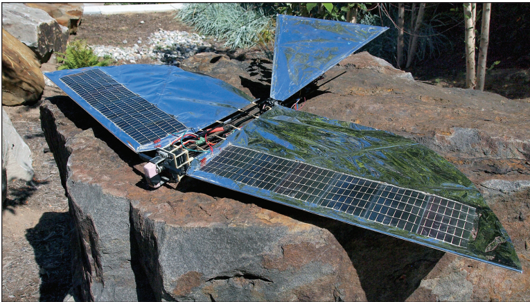
ROBO RAVEN, NOW WITH SOLAR-POWERED WINGS.
