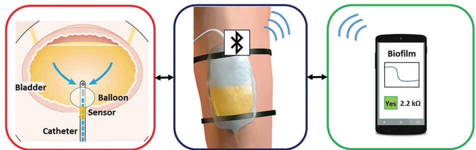
WIRELESS READOUT AND CONTROL SYSTEM SCHEMATIC SHOWING SENSOR EMBEDDED ON AN INSERTED URINARY CATHETER
