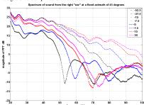
Spectrum of sound from the right "ear" at a fixed azimuth of 45 degrees and different elevations. As the elevation increases, the spectral shape changes significantly.
