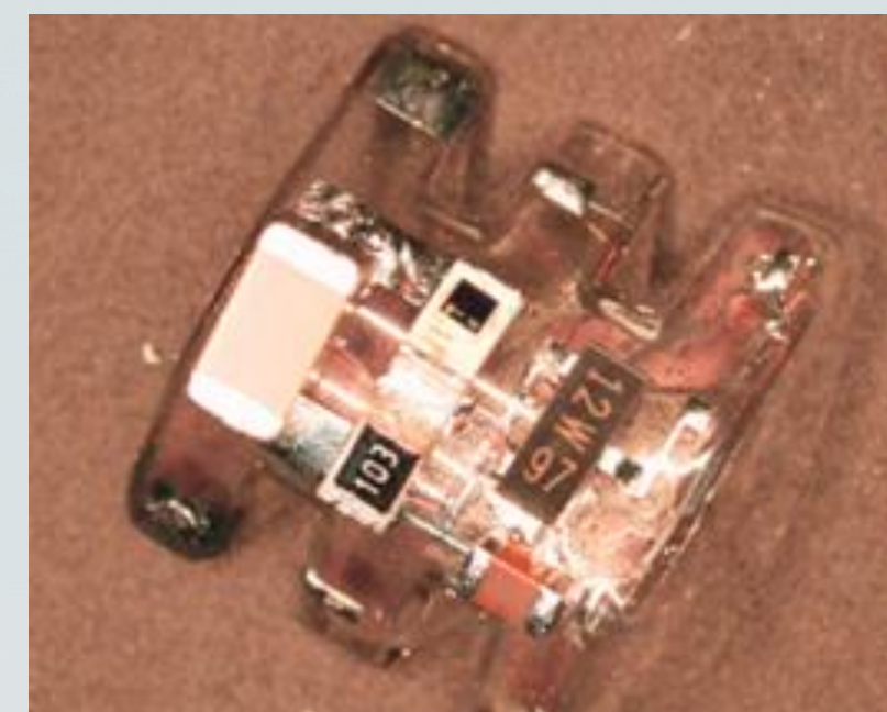
Integration of power and a control circuit for a jumping hexapod (this robot jumped 8 cm!).
