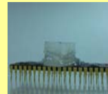
A well is formed on the 40 pin DIP chip to contain the cell medium
