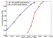
Performance of a R-SPRT based detector using improper training set
