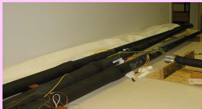
Fig. 2: Gun barrel with mounted sensors
