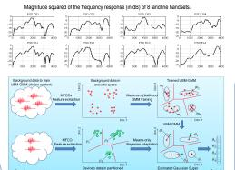
Mechanism to compute the a statistical intrinsic fingerprint of a device
