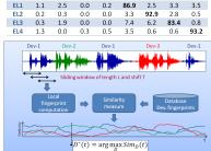
Use of device intrinsic fingerprint to detect multi-device composites
