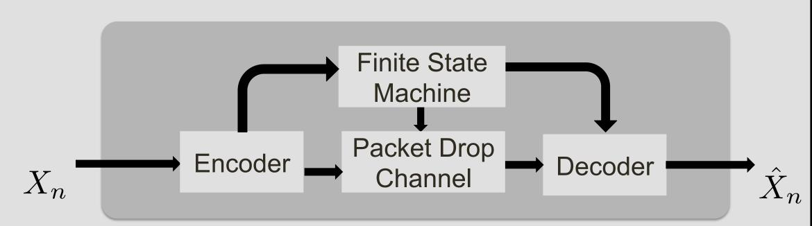
The Finite State Machine state determines the packet drop probability due to channel use.
