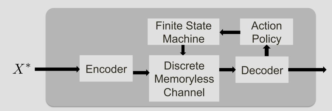
The Finite State Machine state, q, determines the Discrete Memoryless Channel, p(y|x,q).
