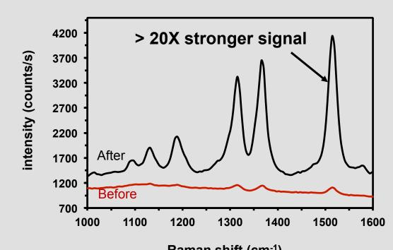
After lateral flow concentration, the signal intensity for Rhodamine 6G (R6G, a common model SERS analyte) is improved by a factor of 20.
