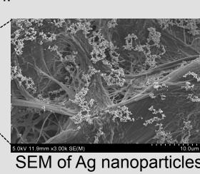
Metal nanoparticles printed onto various paper sensors.
