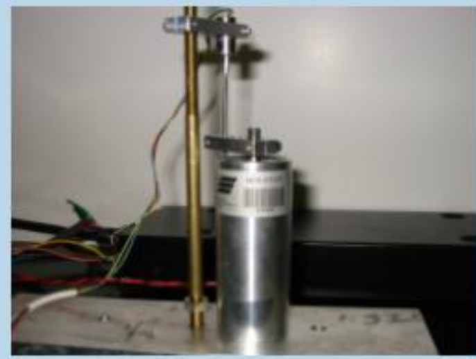
The Terfenol-D actuator and the LVDT sensor
