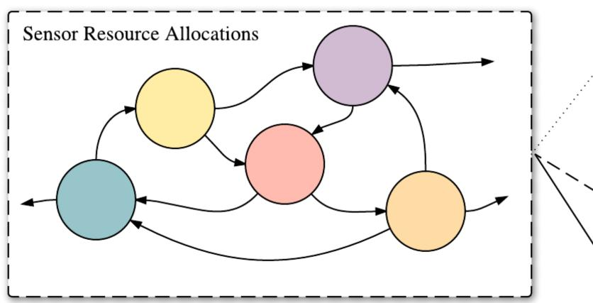
Resource constrained sensor systems with dynamics are modeled by a finite state Markov Process. Each Markov chain state represents a different allocation of resources. Each process is measured over a packet-drop channel with a probability of drop determined by the current resource **allocation**. Applications include:
