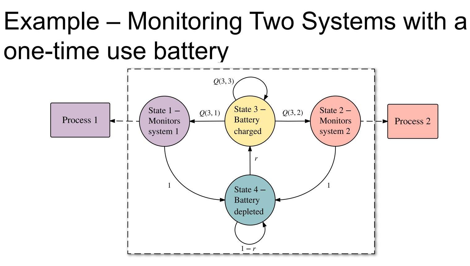
In this example, r is the recharge probability of the battery during a single time step. The transition matrix must be designed to balance when to preserve the battery by not measuring, measure system 1, or measure systems 2.
