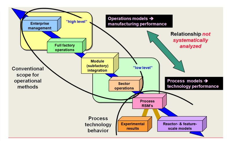
Integrating process models with factory level simulations combines continuous and discrete event simulations to reveal factory-level consequences of changes in processes, equipment architecture, factory capital equipment, and scheduling.
