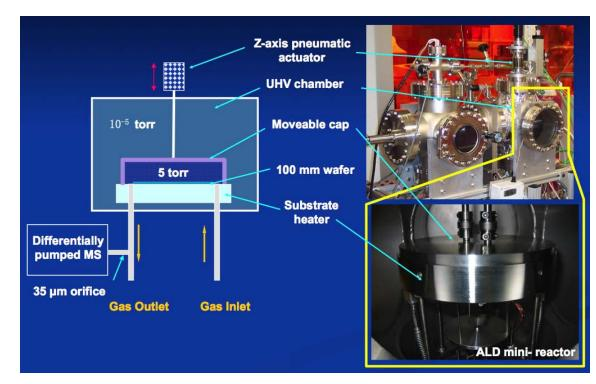
**Real-time, in-situ sensing**, e.g., downstream mass spectrometry, reveals chemical reaction steps and provides metrology for advanced process control (APC).
