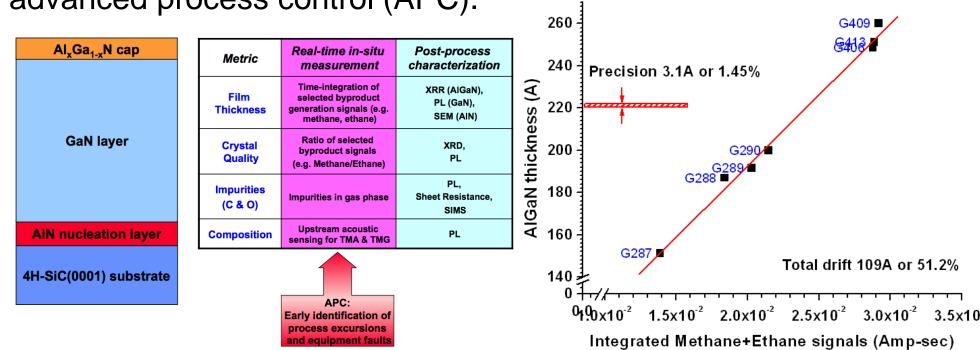
Advanced process control (APC) has been achieved using downstream mass spectrometry in Northrop Grumman's GaN HEMT program, controlling a 20nm AlGaN cap layer to <2% thickness for high speed devices.
