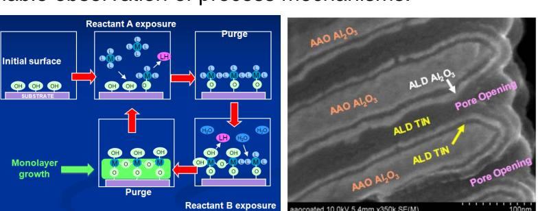
Atomic layer deposition (ALD), providing unprecedented control of materials deposition, one atomic layer at a time even over complex nanotopography, is essential to nanostructure fabrication as sought in NEES, our DOE Energy Frontier Research Center.
