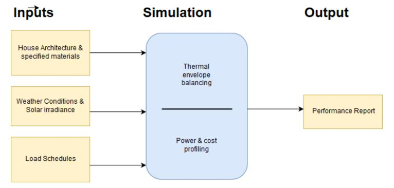
The general schematic of simulation (above) is divided into three parts: inputs, simulation, and output.
