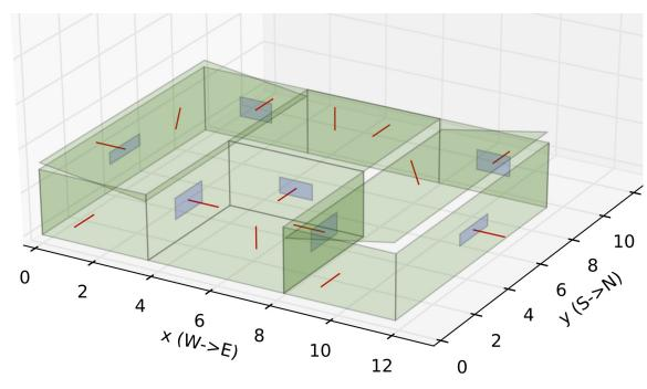
The Virtual House (above) has been designed to use architecture, material properties, weather effects, solar irradiance, and load schedules for input and is simultaneously run among several locations.
