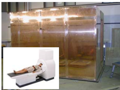
KIT-UMD whole head MEG system & shielded room. 160 axial gradiometers,
