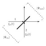
$$\xi_{in}^{-}(t) = \begin{bmatrix} \xi_{a}(t) & 0\\ 0 & \xi_{b}(t) \end{bmatrix} \rightarrow \xi_{out}^{-}(t) = \frac{1}{\sqrt{2}} \begin{bmatrix} \xi_{a}(t) & \xi_{b}(t)\\ -\xi_{a}(t) & \xi_{b}(t) \end{bmatrix}$$
