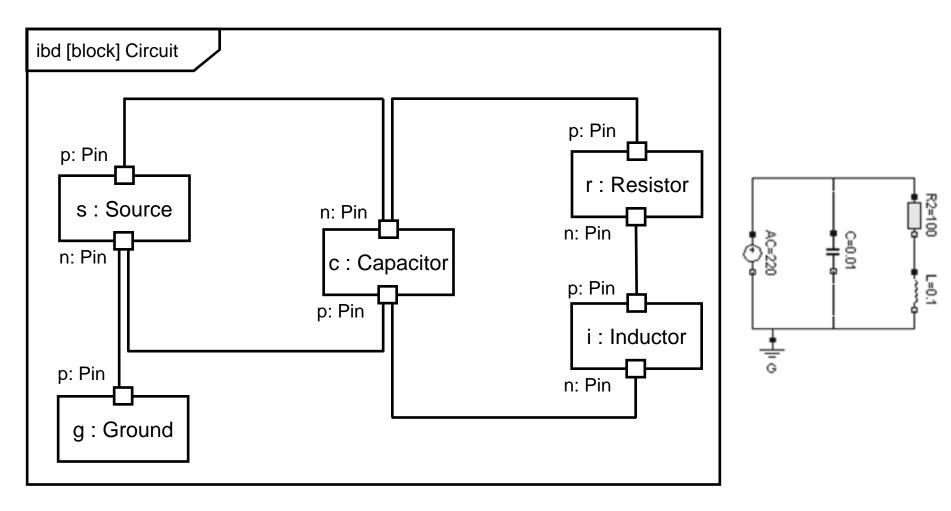
§ N-ary electrical connections broken into binary SysML connectors.
