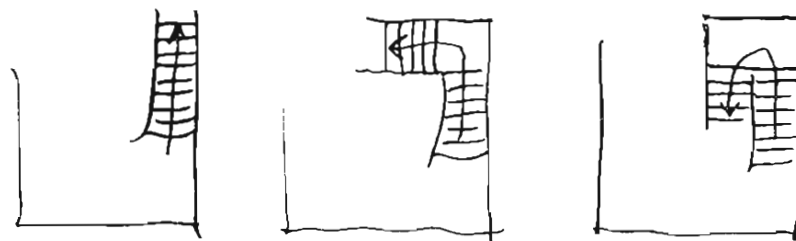
Examples of stair rooms.
