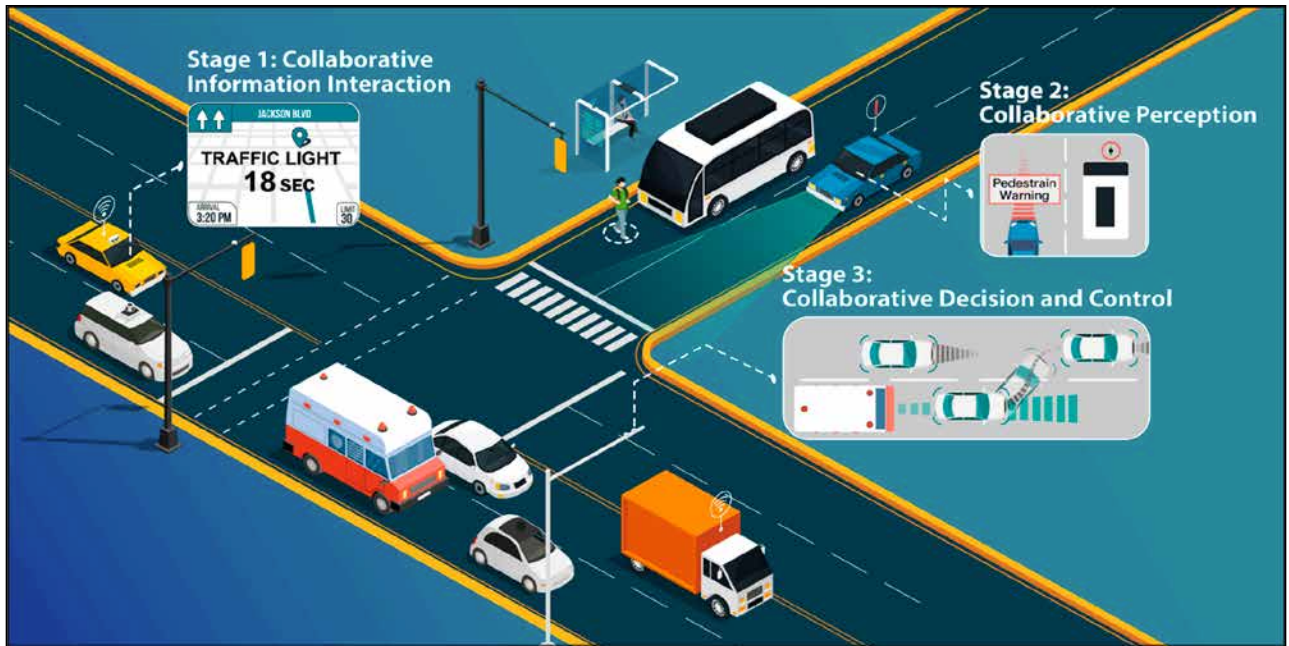
FIGURE 1 Three stages of vehicle-infrastructure coordinated autonomous driving: (1) collaborative information interaction – sensors manage traffic flow and vehicles show drivers and passengers transmitted data (e.g., waiting time at traffic lights); (2) collaborative perception – vehicles gather sensor data (e.g., from roadway cameras) to enhance awareness and safety; and (3) collaborative decision and control – vehicles execute command data (e.g., to make way for an ambulance) to collaborate with adjacent vehicles. Prepared by AIR and Baidu.
