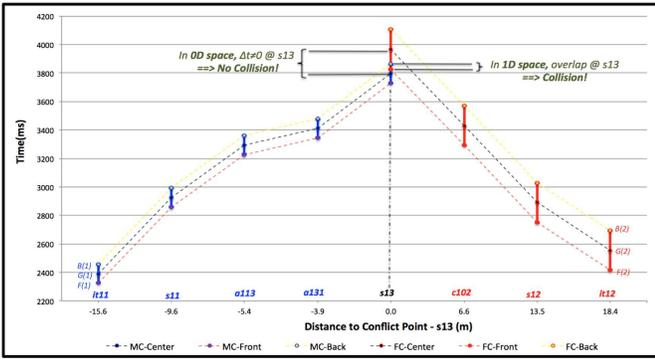
Figure 5. Space-time trajectory for two vehicles on a course of glancing collision.
