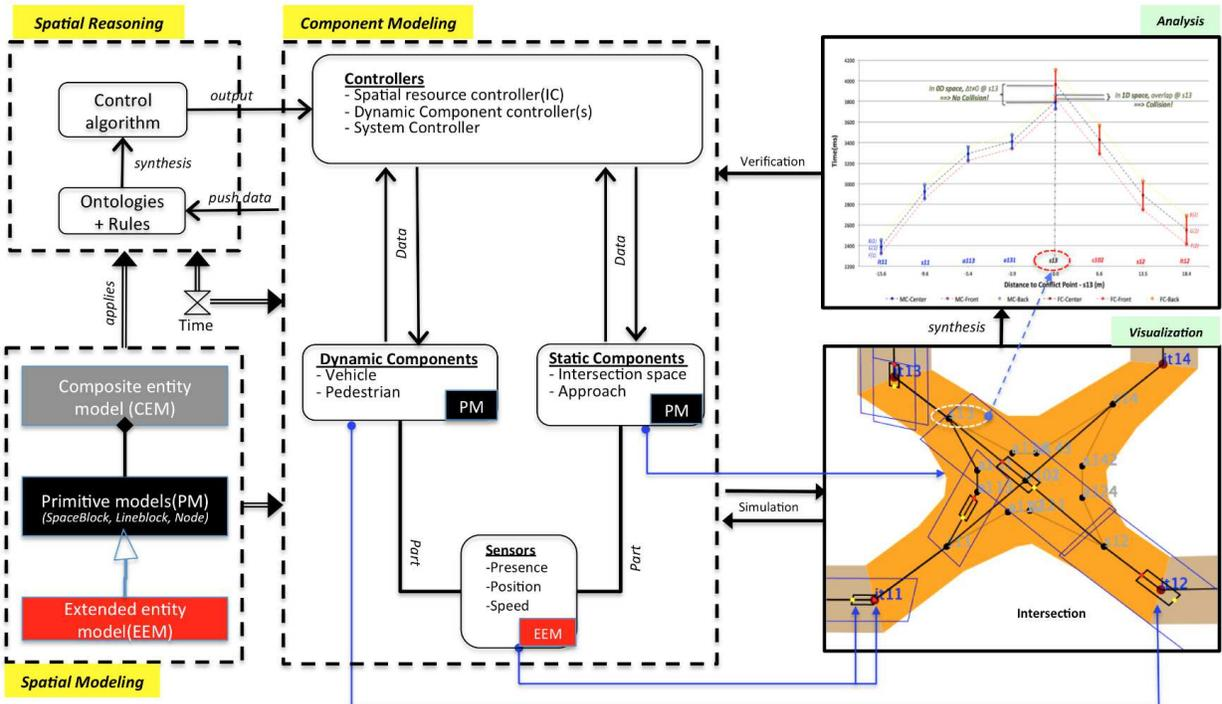
Figure 3. Spatial modeling and reasoning framework extended with views for race track simulation and analysis. The three main elements of the framework are: (1) models of space, (2) models of components, and (3) support for spatial reasoning.
