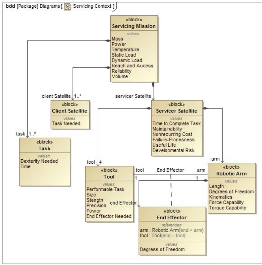
Figure 2: SysML block diagram for Satellite Servicing Architecture.
