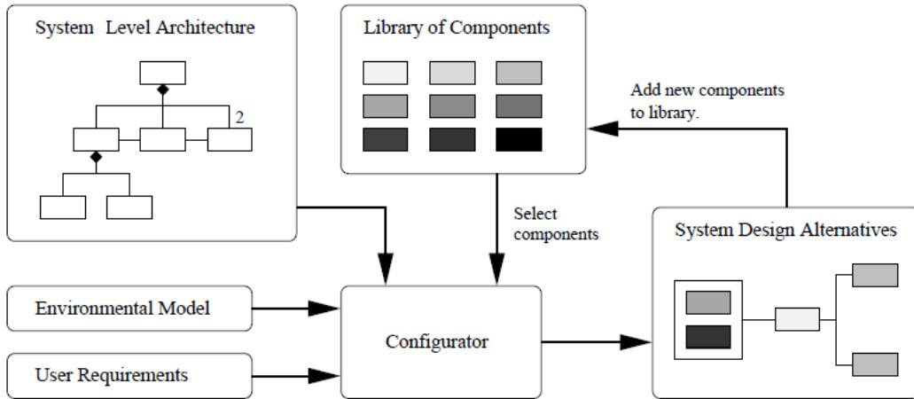
Figure 7: Component-Selection Design Problem (Adapted from Nassar and Austin (2013)).
