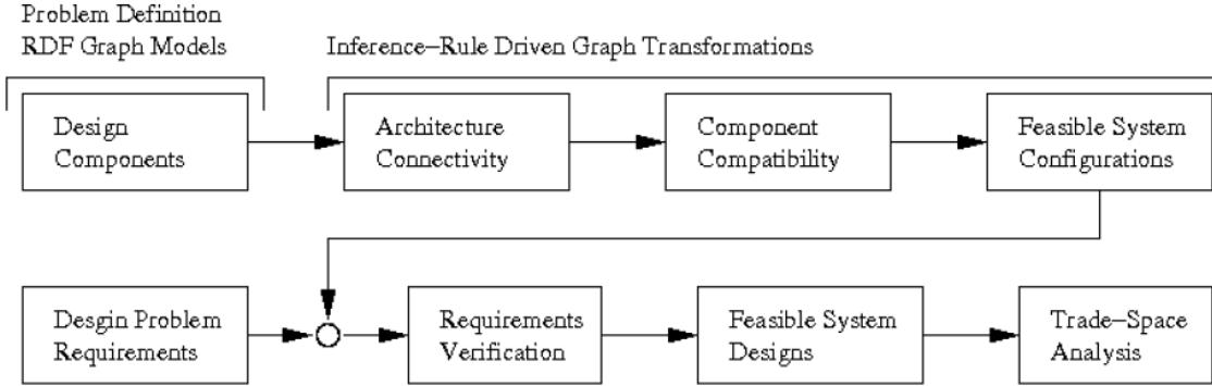
Figure 8: Nassar's and Austin's (2013) Flowchart of Activities for Problem Definition with RDF Graph Models Followed by Inference-Rule Driven Graph Transformations
