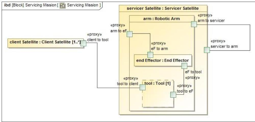
Figure 3: SysML Internal block diagram for Servicing Mission Interfaces and Interactions.
