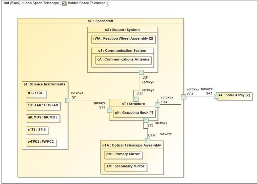
Figure 10: Hubble Space Telescope (HST) System Architecture and Interfaces (as defined on the HST website)
