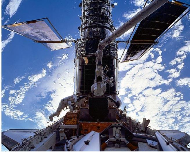
Figure 1: Astronauts Servicing the Hubble Space Telescope (HST) (from the HST website)
