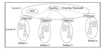
Figure 4.2: Logical Grouping in the Satellite Network Architecture
