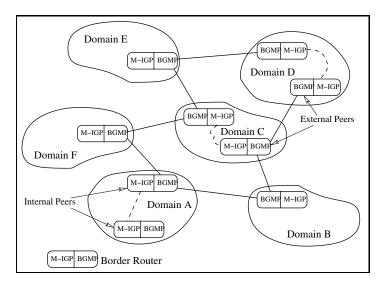
Figure 2.10: BGMP Inter-domain Multicast Architecture
