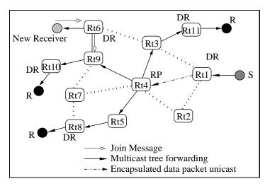
Figure 2.6: Shared RP Tree in PIM-SM. "Join" message for new receiver is sent by its DR towards the RP till it reaches a on-tree router. The DR for source S initially unicasts encapsulated packets to the RP, which de-capsulates the packets and forwards them to all receivers along the shared tree.
