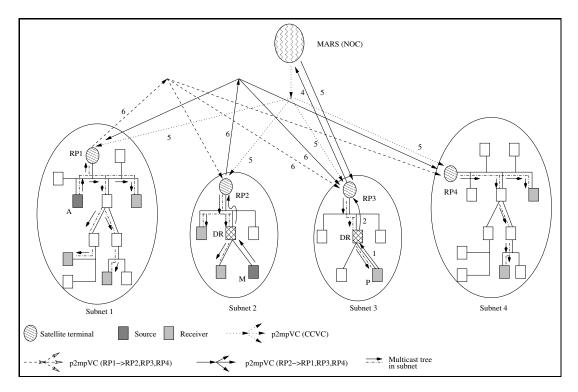
Figure 4.6: Receiver Join to Existing Multicast Group
