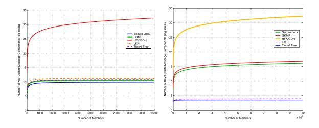
(a) Number of key update messages required for a subnetwork join in Tiered Tree. A subnetwork join in Tiered Tree is equivalent to  $n_2 + 1$  members joining group.
