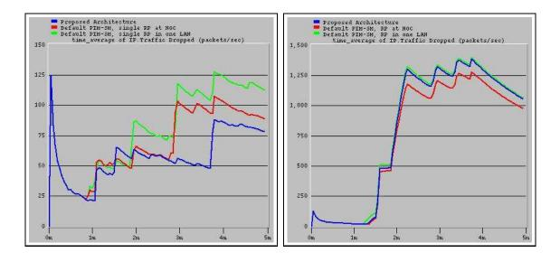
(a) IP Packet Drop for Voice in packets/sec (Y-axis)
