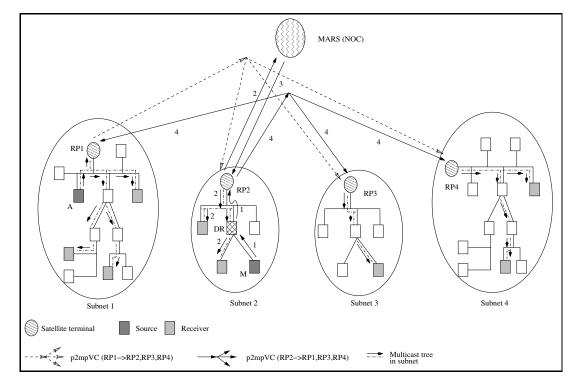
Figure 4.5: Source Join to Existing Multicast Group
