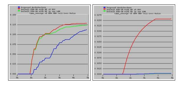
(a) UBR Cell Loss Ratio for Voice Traffic (Y-axis)
