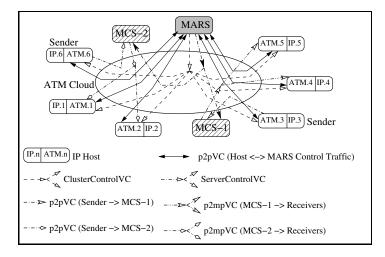
Figure 3.7: IP/ATM Multicast using MARS and MCS
