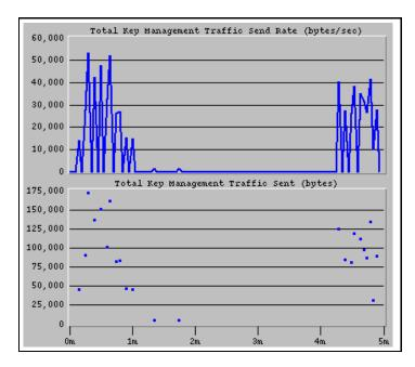
Figure 8.10: Tiered Tree Framework - Many-to-Many: Total Key Management Overhead for All Three Multicast Groups. Top graph gives the send rate in bytes/sec (Y-axis) while the bottom graph shows the traffic sent in bytes (Y-axis). X-axis is the simulation duration in minutes.
