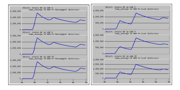
(a) Throughput on the uplinks in bits/sec (Y- (b) VC load on the uplinks in bits/sec (Y-axis) axis)
