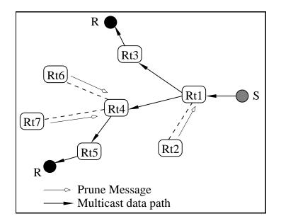
Figure 2.4: RPF Algorithm using Flood and Prune: Routers Rt3 and Rt5 have receivers downstream and accept the multicast data packets. Routers Rt2, Rt6 and Rt7 send prune messages to remove themselves from the SPT for source S.
