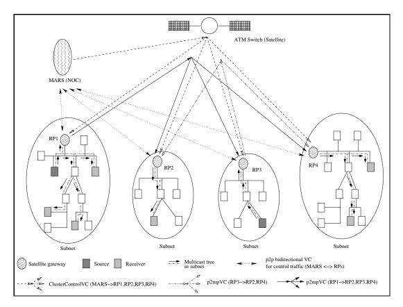
Figure 4.3: The IP/ATM Multicast Framework
