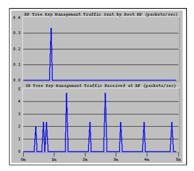
Figure 8.7: Tiered Tree Framework - One-to-Many: Total Key Traffic Received and Sent by Root RP in packets/sec (Y-axis). X-axis is the simulation duration in minutes.
