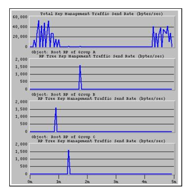
Figure 8.12: Tiered Tree Framework - Many-to-Many: Total Key Traffic vs. RP Tree Traffic for 3 Groups (Y-axis shows the traffic in bytes/sec; X-axis is the simulation duration in minutes).
