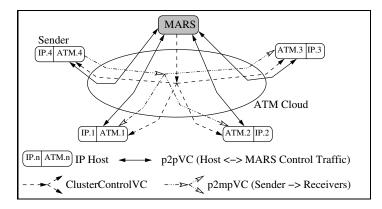
Figure 3.6: IP/ATM Multicast using MARS and VC Mesh
