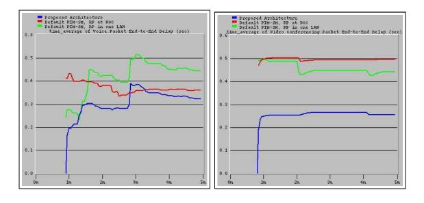
(a) End-to-end Delay for Voice in seconds (Y-axis)(b) End-to-end Delay for Video in seconds (Y-axis)
