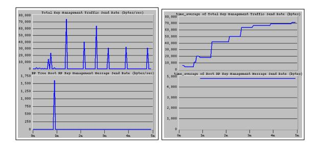
(a) Total Key Traffic Sent vs. RP Tree Traffic(bytes/sec; Y-axis)
