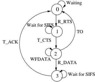
Figure 2: FSM representation of the receiving node.
